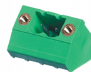
pitch 5/5.08 mm from 2 to 23 poles 45° version locking screw flange
